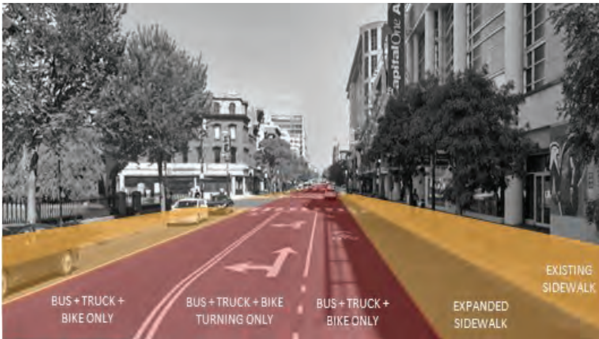
Figure 2I: Diagrams depicting initial DDOT ideas for bus-priority lanes on 7th Street and the overall circulation concept.
