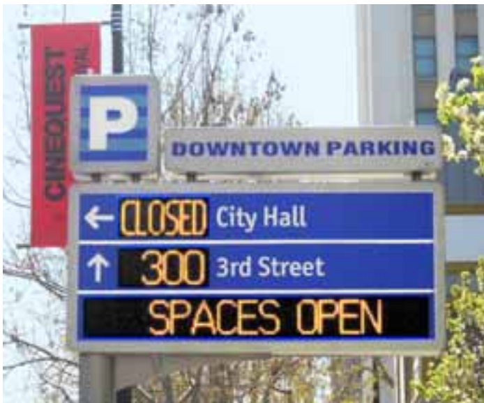
The City of San Jose, California, has invested in real-time parking availability and wayfinding infrastructure. PHOTO COURTESY OF TCS INTERNATIONAL, A PARKING AND TRANSPORTATION MANAGEMENT SYSTEM INTEGRATOR.
